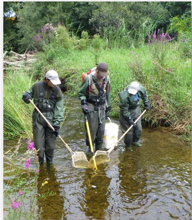
MVCA staff using a backpack electro-fishing unit with two people prepared to net fish
