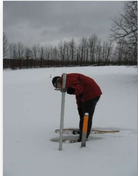
Measuring snow depth and equivalent water content
