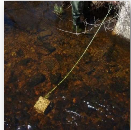
Deploying a temperature logger
