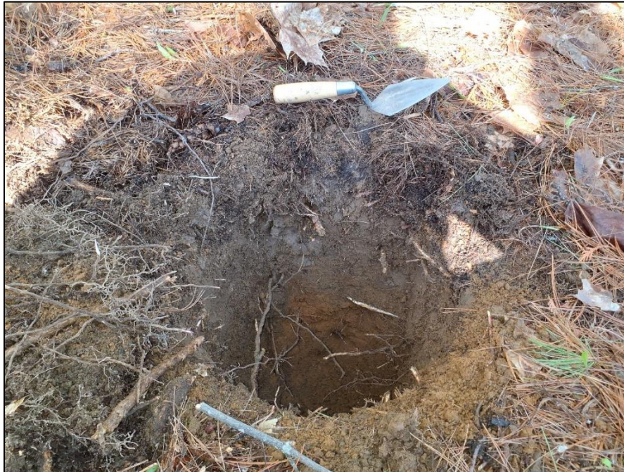
Image 26. View of sample test pit in the western portion of the southern study area showing natural soil stratigraphy, facing west. (PR23-021D078)
