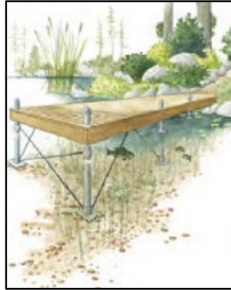
Removable Pipe Dock
