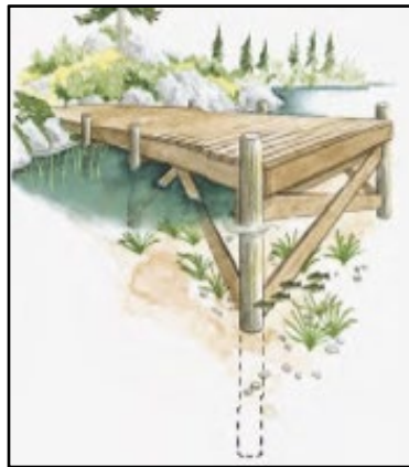
Permanent Post Dock
