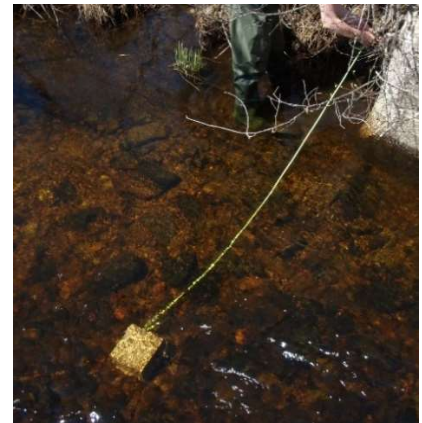
Deploying a temperature logger
