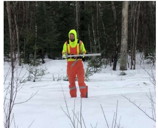
Measuring snow depth and equivalent water content
