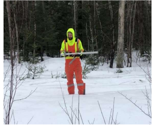
Measuring snow depth and equivalent water content
