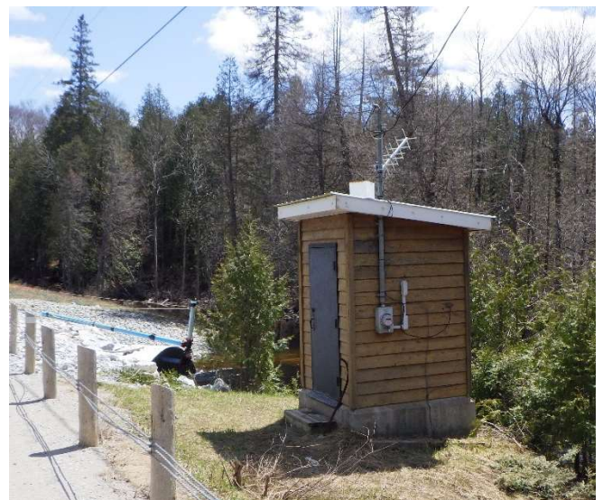
The stream flow and rain gauge station on Buckshot Creek near Plevna.
