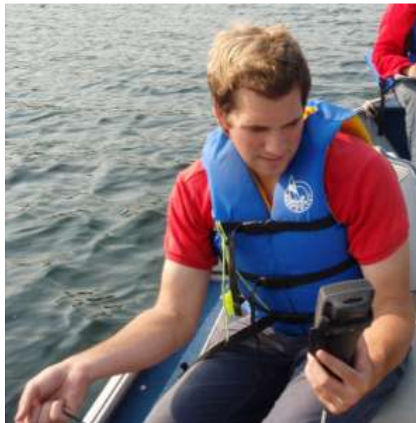
The Dissolved Oxygen Metre is used to gather DO and temperature readings. The probe is lowered into the lake and readings are taken at every metre from the hand-held screen.
