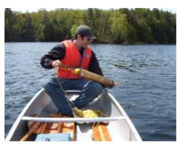
The Kremmerer Bottle (pictured above) is used for sampling water at specific depths. The bottle is lowered with both ends open to the required depth, a weight (on the rope) is dropped, when the weight hits the bottle the it causes both ends to close sealing the sample water in the bottle.
