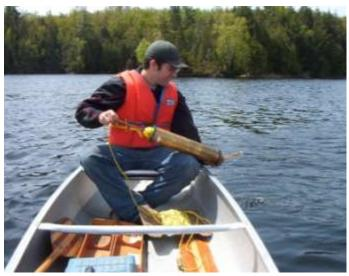
The Kremmerer Bottle (pictured above) is used for sampling water at specific depths. The bottle is lowered with both ends open to the required depth, a weight (on the rope) is dropped, when the weight hits the bottle the it causes both ends to close sealing the sample water in the bottle.
